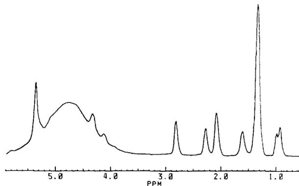
**Figure 3.**  $^1\text{H}$  MASS spectrum of a single bean (variety black turtle) showing substantial amounts of adsorbed moisture giving rise to a broad resonance centered around 4.8 ppm. Oil contains linolenic acid contributing to characteristic peak at 0.98 ppm.
