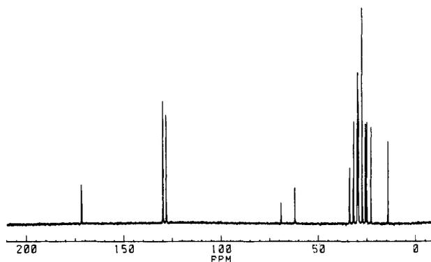
**Figure 4.**  $^{13}\text{C}$  spectrum of a single sunflower seed as obtained within 15 min. Since magic angle sample spinning reduced inhomogeneous line broadening, the resonances show remarkable resolution and sensitivity.
