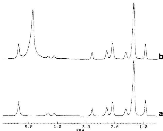
**Figure 1.** (a) Typical  $^1\text{H}$  MASS spectrum of a single sunflower seed. All resonance peaks are assigned to liquidlike oil, and they facilitate nondestructive characterization of oil composition. The signal at 2.78 ppm determines the amount of linoleic fatty acid. (b) Spectrum of the same seed after soaking in water for 30 min.
