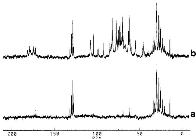
**Figure 5.** (a) MASS  $^{13}\text{C}$  spectrum of a single bean showing oil as the only liquidlike component. (b) Spectrum after soaking in water, which starts germination process and makes signals of dissolved carbohydrates and proteins observable.
